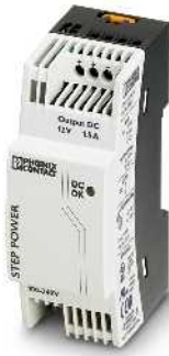
Power supply, 1 AC, 12 V DC, 1.5 A NEC Class 2
